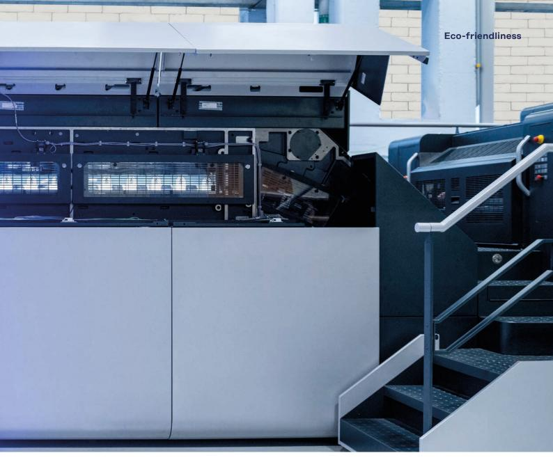
It starts with the VariDry dryer family: The VariDry<sup>Blue</sup> IR/TL dryers in delivery and delivery extension combine maximum drying performance with low energy consumption. By reusing the recirculated air as drying air, we reduce the energy requirements compared with conventional dryers several times over. This has an impact on the entire printing process, as drying usually involves the highest electricity consumption.
