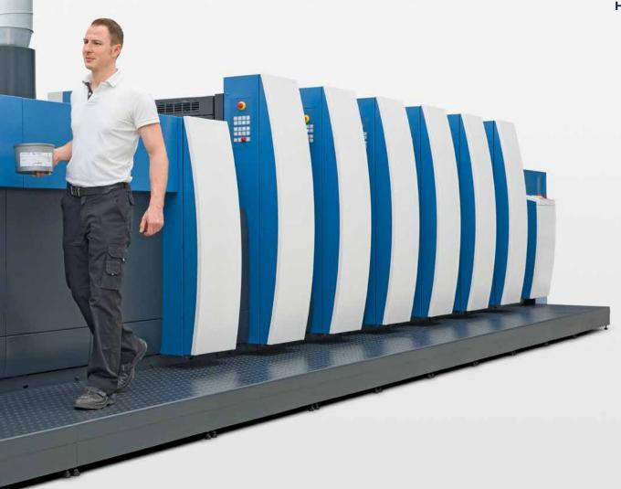
As if that were not enough, the Rapida 75 PRO stands out with a new operating concept. The ErgoTronic console with Touch-Tronic control is now also standard for the small Rapida presses, eliminating the previous distinction between a delivery display for press operation and a console for job management.
