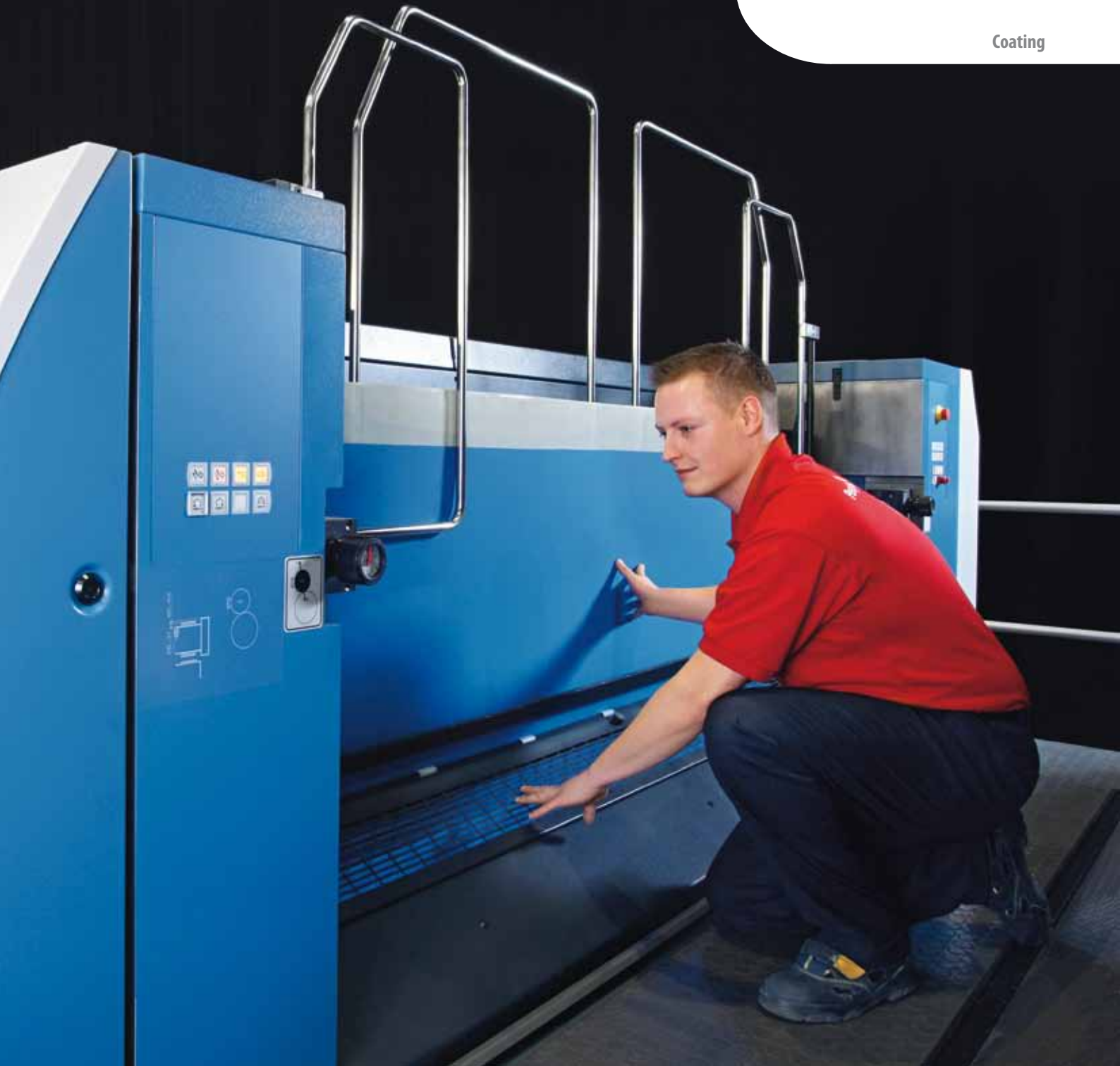
Automated functions permit fast coating plate changes
