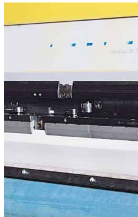
Split rear clamping bars facilitate any manual register corrections
