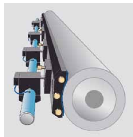
Anilox roller with chambered doctor blade
