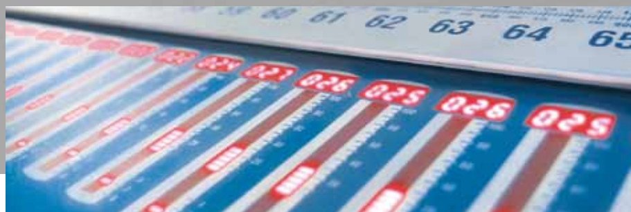
Zone-by-zone ink profile settings at the control console
