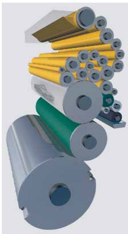
Schematic representation of the inking unit
